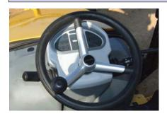
Steering wheel with a knob for easy maneuvering and front dash with critical warning lights.
