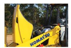
A tiltable engine hood allows access to service check points and can be locked with the ignition key.
