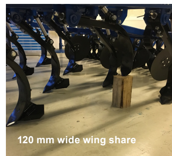
Tri-Max NSH with 2 D tines and 50x20 mm point
