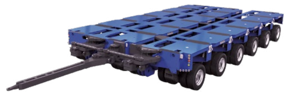
BEST PERFORMANCE CAPABILITY FOR ANY LOAD Due to the extensive range of accessories, the THP/SL heavy-duty modules can be flexibly adapted to the specifications of the load, as shown here with a parallel combination (1+1/2).
