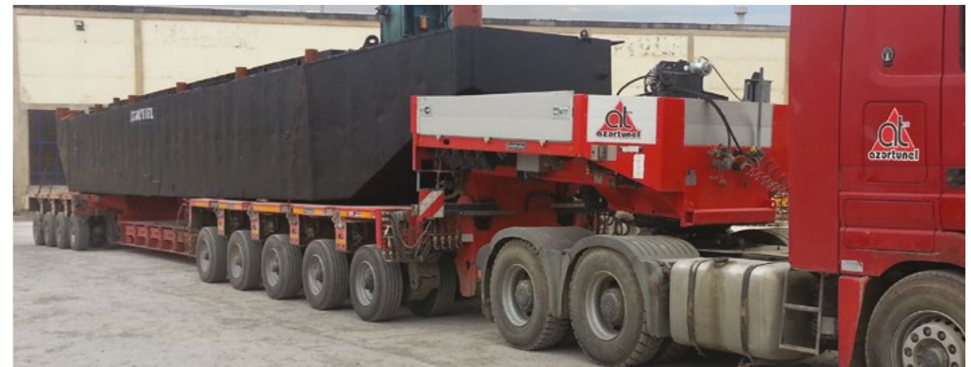
APPLICATION EXAMPLE THP/SL-S (5+4) transporting a steel component. Accessories such as excavator bridges can be used flexibly, also to extend the loading area as in this example.
