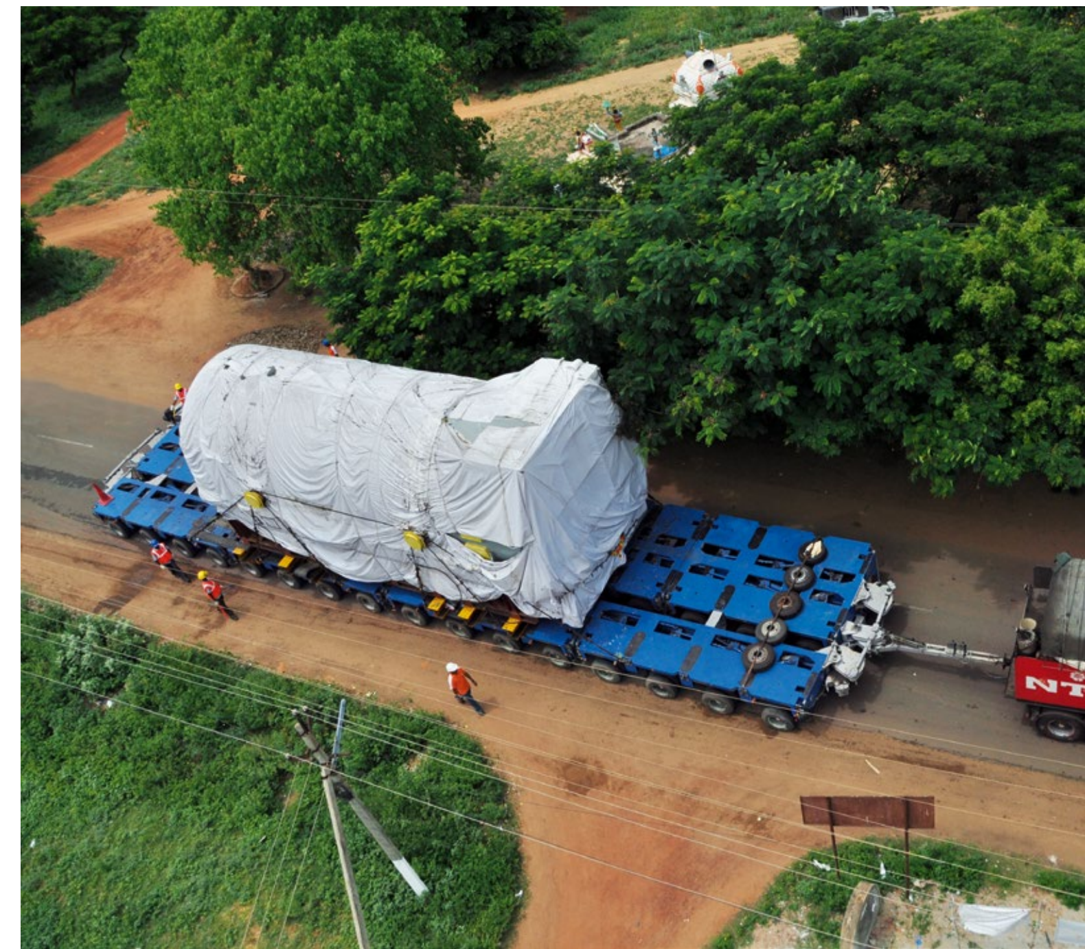
BEST PERFORMANCE CAPABILITY FOR ANY LOAD Due to the extensive range of accessories, the THP/SL heavy-duty modules can be flexibly adapted to the specifications of the load, as shown here with a parallel combination (1+1/2).
