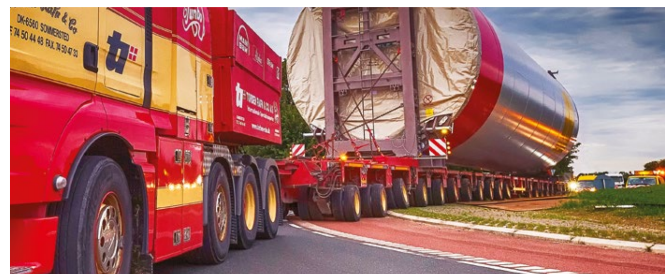
FLEXIBLY COMBINABLE Transport of a steel tower segment for an offshore wind turbine on a 22-axle THP/SL combination.
