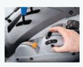
The advanced EDC controls are ideally placed to fine-tune drop rate, the height limiter, sensitivity and slip for uniform cultivation and maximum traction.
