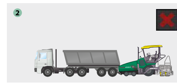
Stop: Lorry must halt. It has docked.
