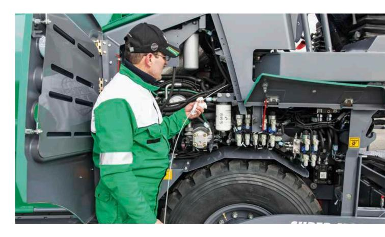
The identical servicing concept of the "Dash 3" pavers permits rapid, uncomplicated maintenance. All servicing points on the machine are easily accessible via large hinged panels.
