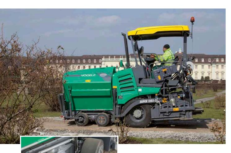
A powerful paver that's a comfortable drive on the road. The precise steering and handling characteristics make for the SUPER 1303-3i's excellent manœuvrability, as demonstrated by its outside turning radius of just 4.9m (3.8m with "Pivot Steer"). With its powerful traction drive, the machine can pave swiftly and travel on public roads at a maximum speed of 20km/h. So if its next job site is close at hand, there is no need for a low-bed trailer to transport the paver.
