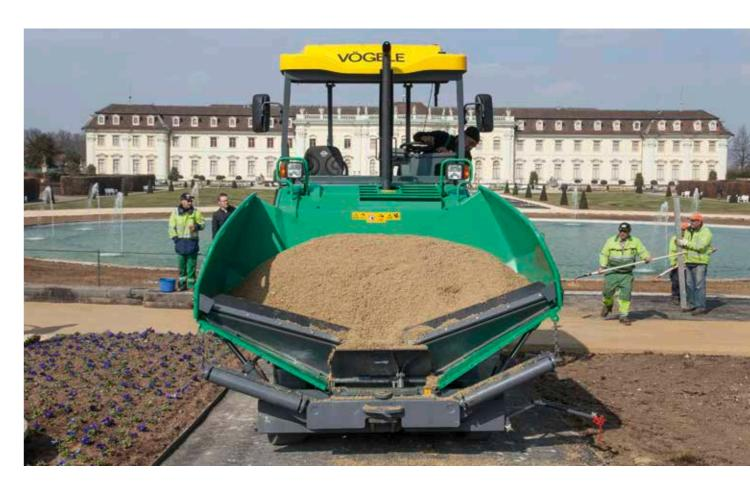
Despite the paver's slim profile, its material hopper holds 10t. The hydraulic hopper front (option) supports both supply of the paver with mix and emptying of the material hopper. The paver comes with oscillating push-rollers to ensure the shock-free docking of feed vehicles.
