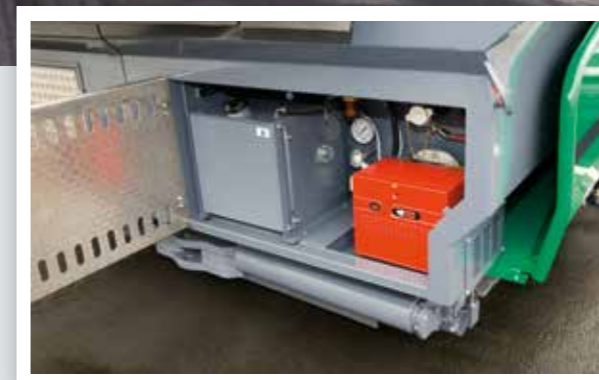
A heating unit (diesel fuel) featuring a heating capacity of 30 kW maintains an ideal emulsion temperature.
