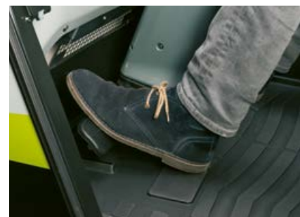
The brake pedal with inching function reduces fuel consumption and brake wear.
