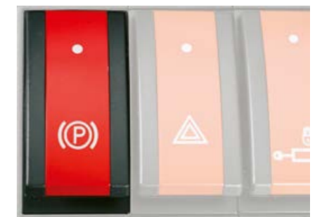
The toggle switch allows the parking brake to be operated manually.
