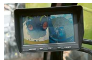
The images from the front and rear cameras are transmitted to the monitor in the cab.
