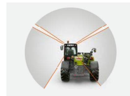
Unobstructed view to the rear for safer work, thanks to the low-mounted telescopic arm.
