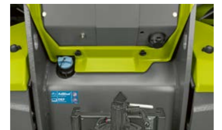
Easily accessible AdBlue filler neck for efficient exhaust gas aftertreatment.
