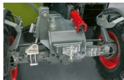
Greater off-road safety thanks to hydraulic levelling.
