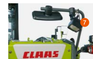
Halogen lights on the rear mirror bracket for illuminating the rear of the machine:
