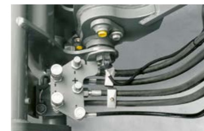
Well-protected hydraulic connections on the implement carrier.
