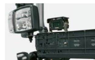
A high-resolution camera at the front right provides clear images even in twilight conditions.
