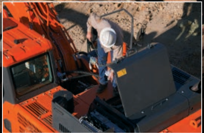
Easy access to regular inspection points
