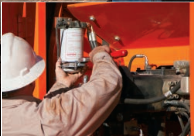
Ground level access to all filters
