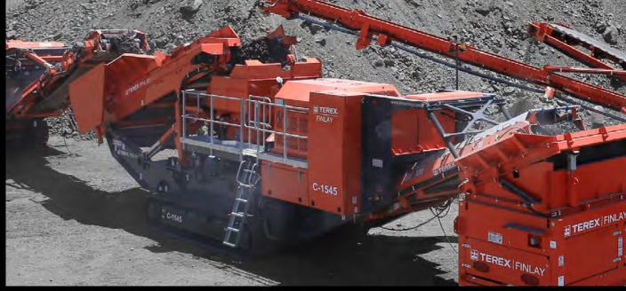
The Terex® Finlay C-1545 is a high capacity and aggressive cone crusher that consistently provides high output capacity and a product with excellent cubicity. This efficient and productive machine incorporates the NEW Terex® 1150 cone crusher driven by direct clutch drive with variable speed, automatic tramp relief and hydraulic closed side setting (CSS) adjustment.
